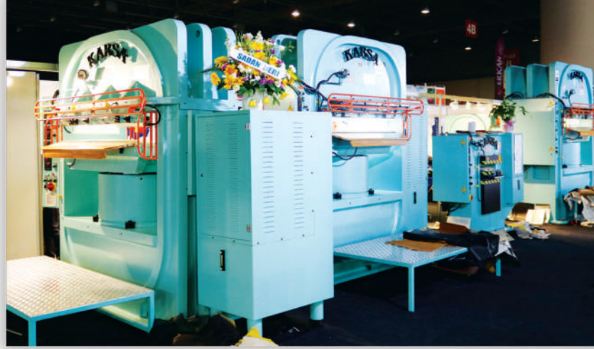
SAYA PRESİ (SHOE-UPPER PRESS) KM-300 212 TON 300 BAR 450mm*450mm
