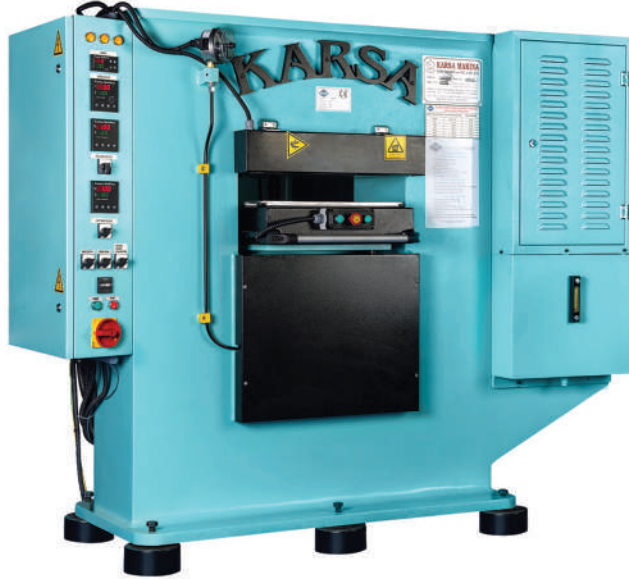
SAYA PRESİ (SHOE-UPPER PRESS) KM-300 212 TON 300 BAR 450mm*450mm
